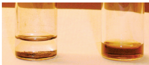
Figure 6. Photograph comparing dispersions of polymer-II-coated Co nanoparticles subjected to no UV irradiation (left) and UV irradiation (right) after rinsing by \text{CHCl}_3 thrice.
